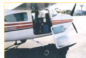
CSU's multispectral airborne imaging system. 4-bands: NIR (770 nm), R (650 nm), G (550 nm), B (450 nm)
